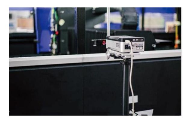
•A Marble test is performed to measure theXand Y axis, calculating any necessary adjustments to ensure perfect level and alignment along length of machine.
