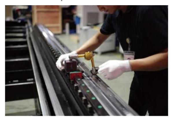
• A collimator is run along the fulllength of the guide rail, testing for straightness. Adjustments are made as required to ensure linear accurate linear accuracy.
